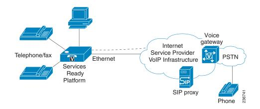
The ATA maintains the state of each call and makes the proper reaction to user input events (such as on/off hook or hook flash). Because the ATA uses the Session Initiation Protocol (SIP), it is compatible with most Internet Telephony Service Provider (ITSP) offerings.
